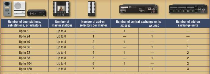
**NOTES:** Use the AX-248C for systems with more than 4 master stations (may change the required quantity of AX-320Cs). Two PS-2420UL power supplies are required per system.
